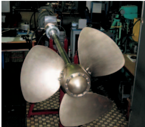
Fig. 1. Low-power CP propeller placed at the Faculty's laboratory test stand
