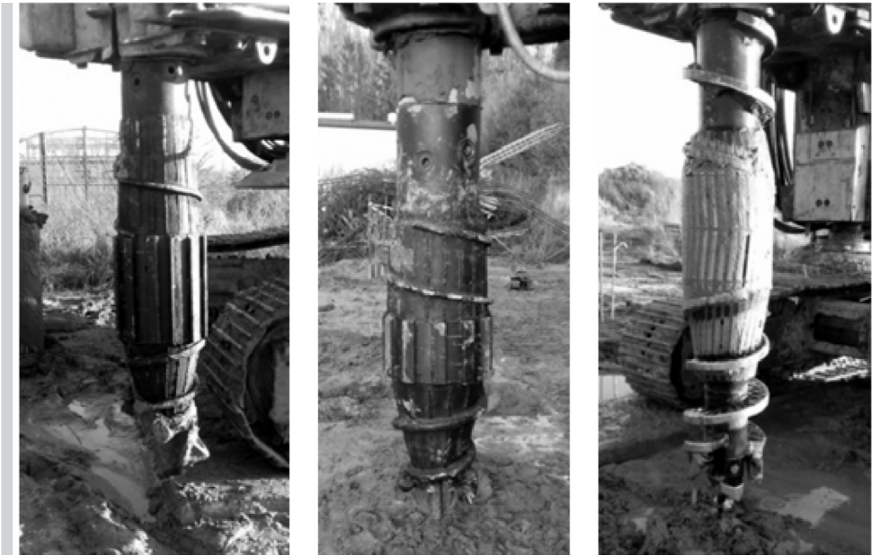
Figure 2. Displacement pile augers tested in the research project: a) DPDT auger, b) DPDT-S auger (shortened length version), c) SDP auger, [6]
