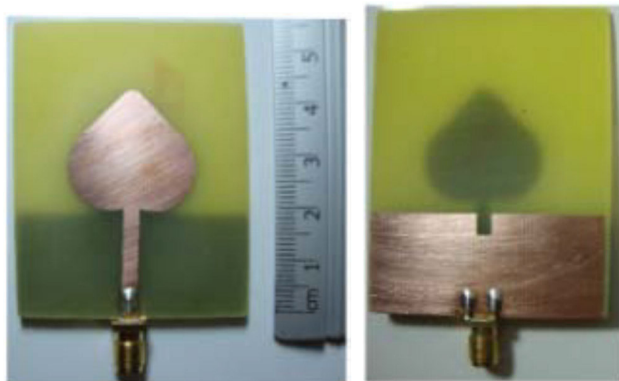
FIGURE 11. Cotton leaf-shaped printed monopole antenna (a) The top side and (b) Lower side of the fabricated antenna [61].
