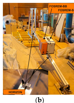
Figure 11. Modified shaking table: (a) scheme (top image) and trigonometric dependence for Equation (9) (bottom image: H = 0.5 \text{ m} , L = 3.7 \text{ m} ); (b) general view of shaking table with mounted FOSREMs and HZ1-100-100.
