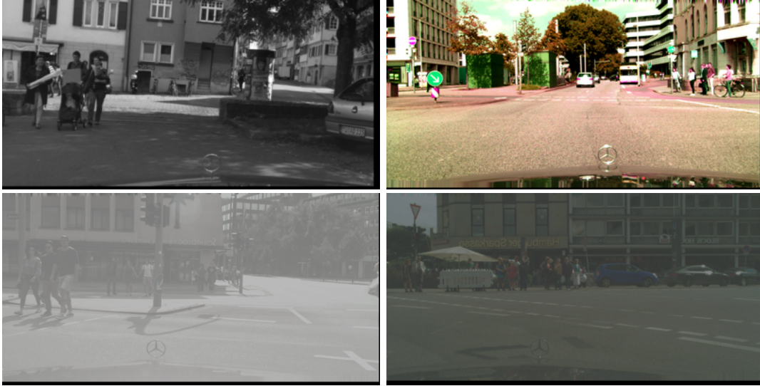
Figure 4.1: Examples of augmented images: color drop (top left image), color distortion (top right), overexposed image (bottom left), gaussian noise (bottom right).
