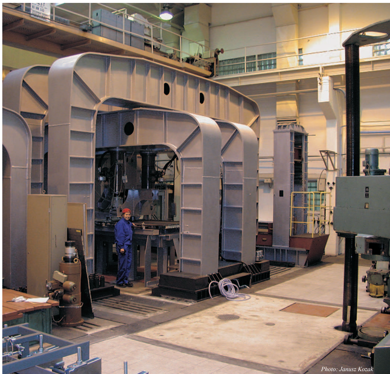
Versatile stand for strength tests of natural scale ship hull units, Faculty of Ocean Engineering and Ship Technology, Gdańsk Technical University .
