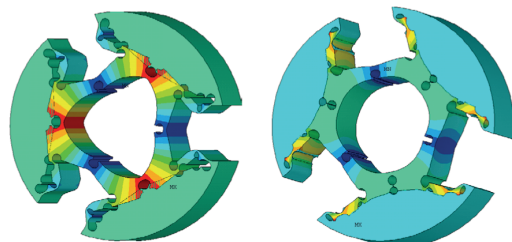
Fig. 21. W9-w version of bearing – examples of a useful modal shape at the frequencies of 7.3 kHz (to the left) and about 27 kHz (to the right)
