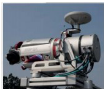
Fig. 2. Riegl VMZ-400 Horizontal mounting [5].
