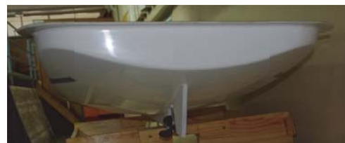
Fig. 9 Model without appendages during the test
