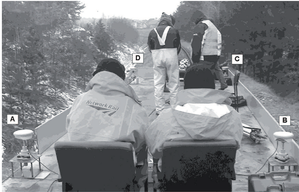
Fig. 6. GPS Total station receivers location on the platform (trials in 2009)
