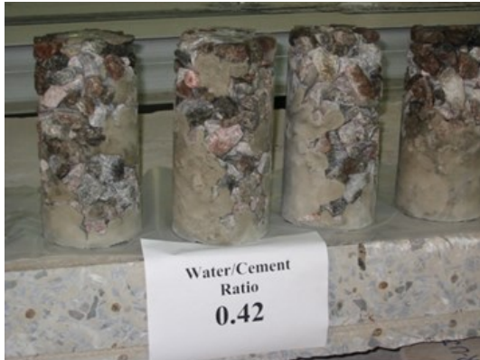
Figure 2. Shown grout was not able to fill all the voids in the aggregate skeleton.
