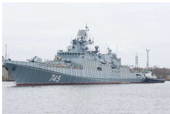
Fig. 1. Admiral Gorshkov-class frigate during demagnetization [7].
