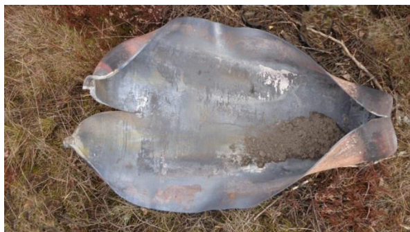
Fig. 5 Fully ruptured acetylene cylinder
