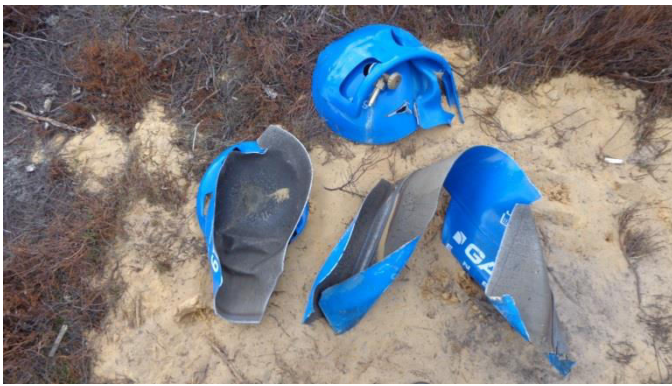
Fig. 19 Shrapnel created during the blow of LPG cylinder (all debris gathered together)
