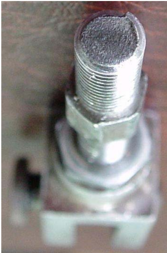
Fig. 3. A view of the fatigue fracture with marked zones of conducted fatigue damage
