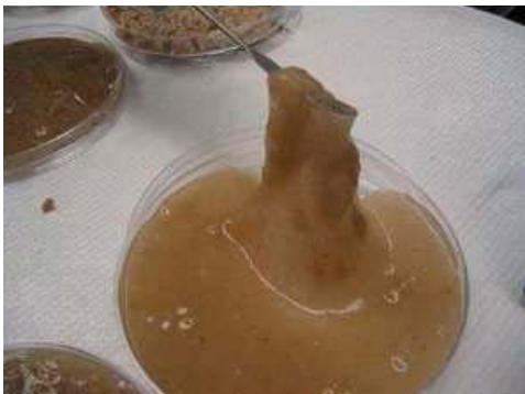
FIGURE 1. Biopolymer – sand viscous mixture (Knox and Petriso 2010)
