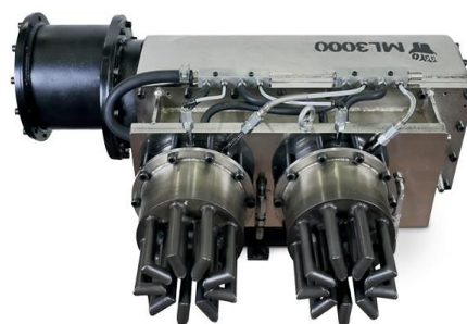
Fig. 1. Two-cylinder Stirling engine Genoa, ML3000, power 3 kWe [13]
