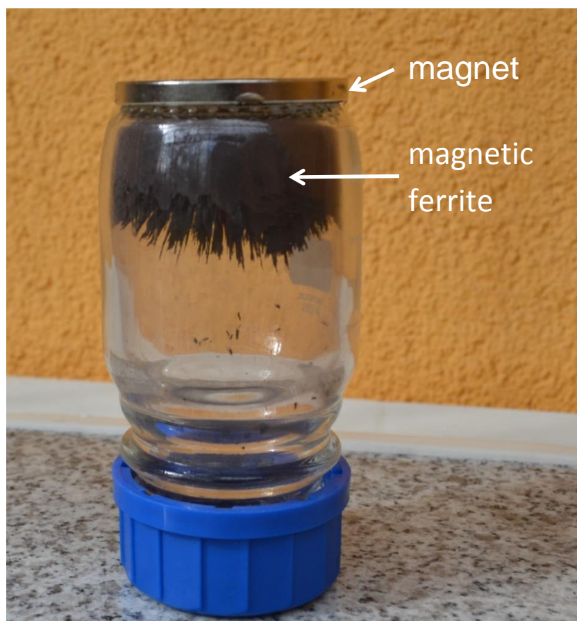
Fig. 3. The magnetization of the nickel ferrite nano-particles in the magnetic field of the permanent magnet.
