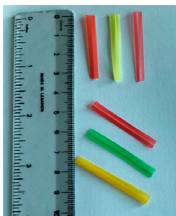
Figure 1. Shredded waste plastic straws (WPSs).
