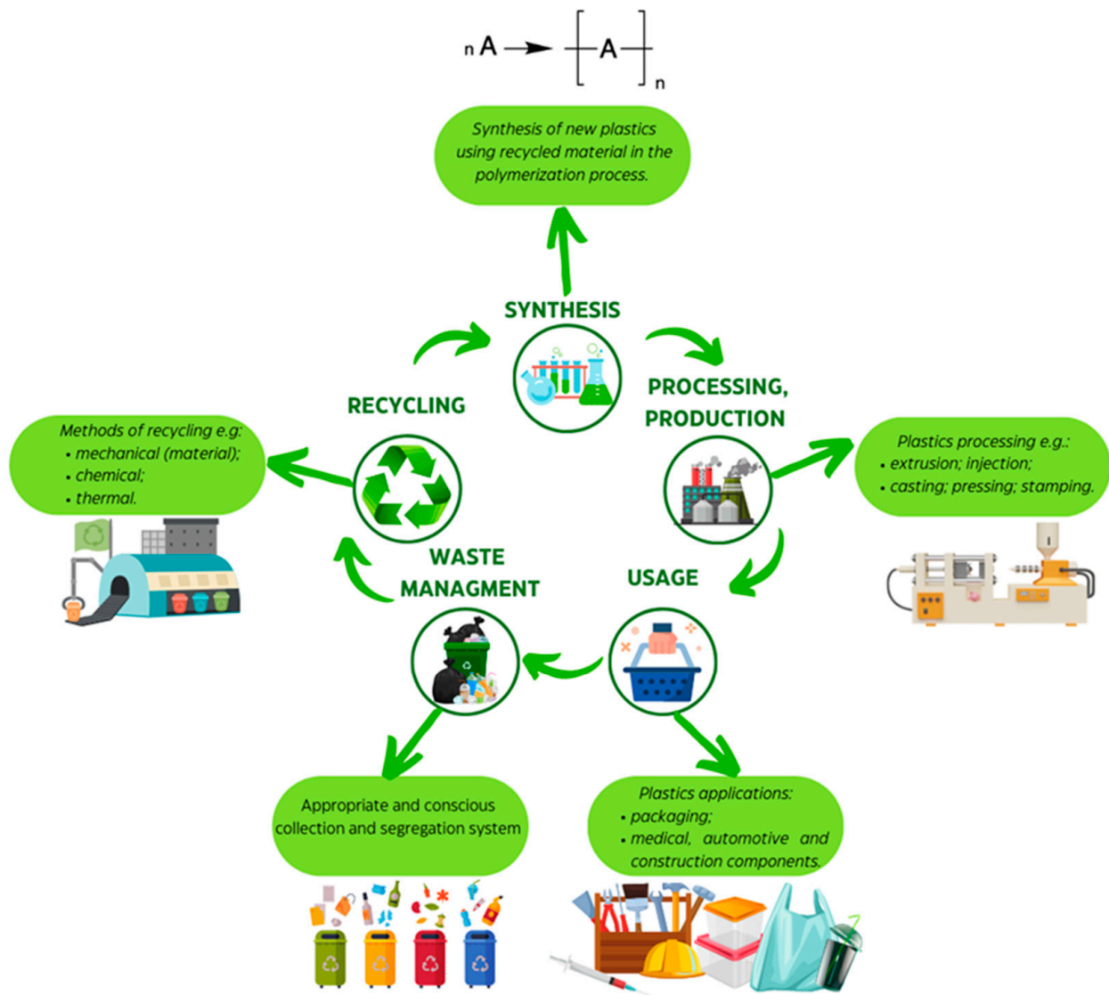
Figure 1. Scheme showing the circular plastics life with selected examples of processing or operation at each particular step. The life of circular plastics represents a sustainable model in which plastics remain in circulation for a longer period through their reuse and recycling [11].
