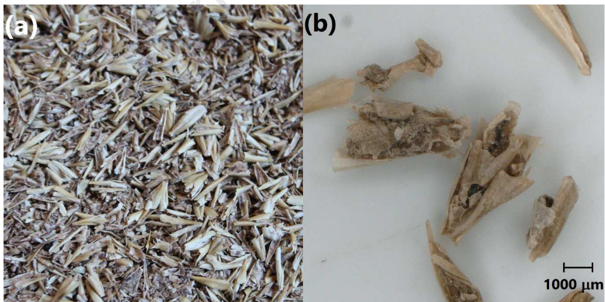
141 Figure 1. Macroscopic (a) and microscopic (b) appearance of applied BSG before extrusion grinding.
