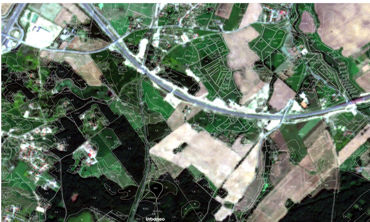
Figure 7. The Stawiguda land use parcels overlaid on an image obtained from a Sentinel-2 satellite on 26.08.2019. The new road and other recent investment activities are properly represented.
