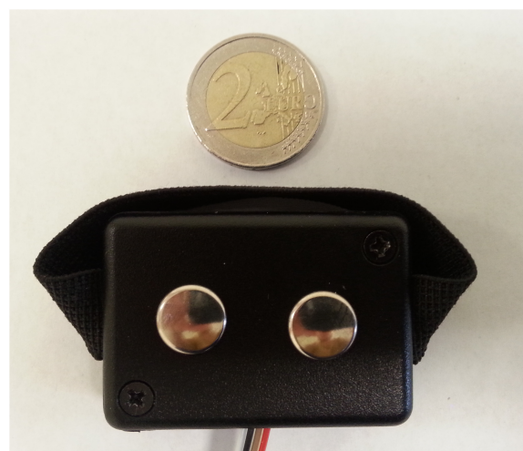
Fig. 5. Skin conductance sensor.
