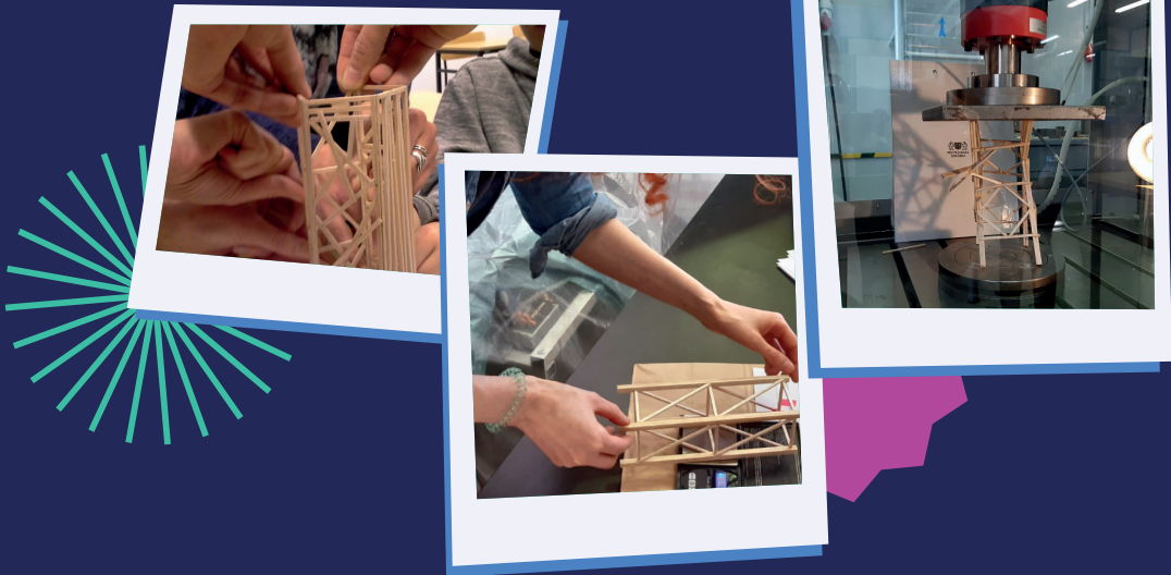
Balsa wood structures built by students during a traditional class are then tested with loading equipment.
