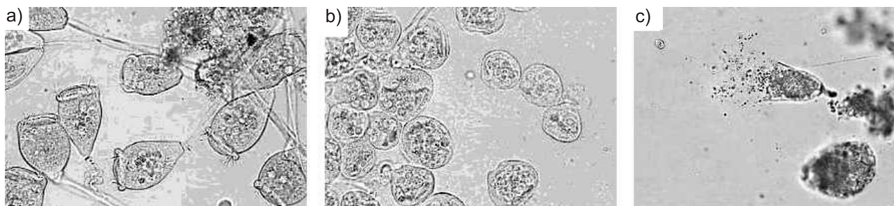
Fig. 6. Microscopic images of activated sludge protozoa (magnification 400 \times ): a) control sample, b) and c) sludge with LAS load 25.6 mg·(g·dss) -1 .
