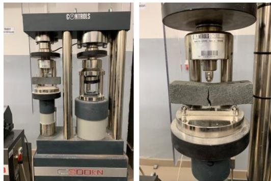
Figure 4. Flexural strength test [Fot.Y.Gu].
