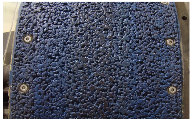
Fig.8. SMA8 surface replica (own material)
