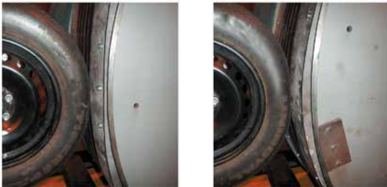
Fig. 4. Minimum (left) and maximum (right) dynamic deflection of the tyre rolling on the sinusoidal replica road surface
