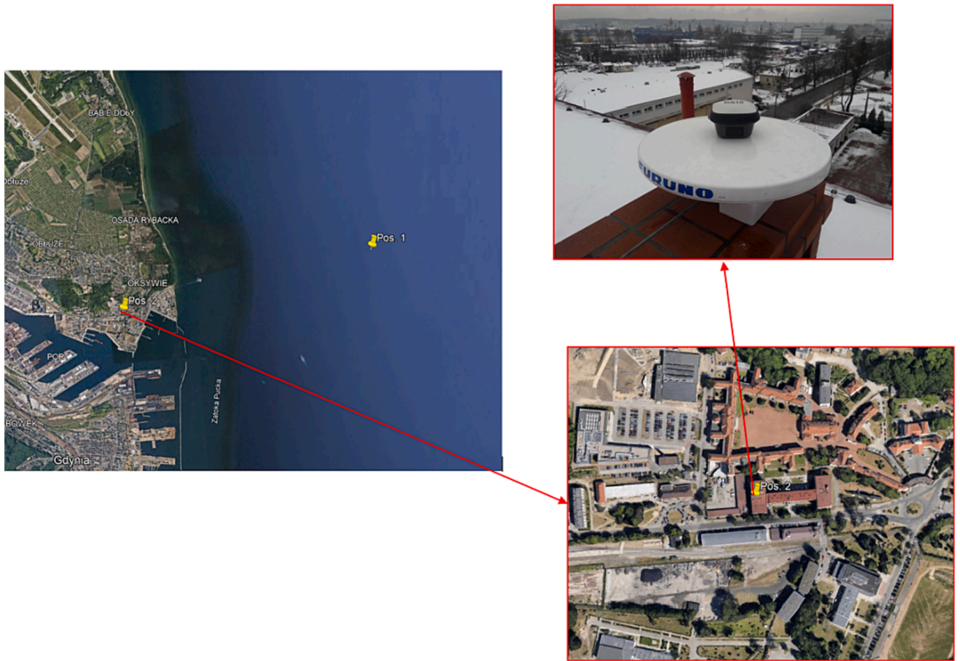
Fig. 7. Satellite images with marking of survey positions for static mode (Pos.2) and dynamic mode (Pos. 1) measurements, and a photo of the Furuno GPS antenna placed on the roof together with the antenna of the Leica GPS-RTK reference receiver.
