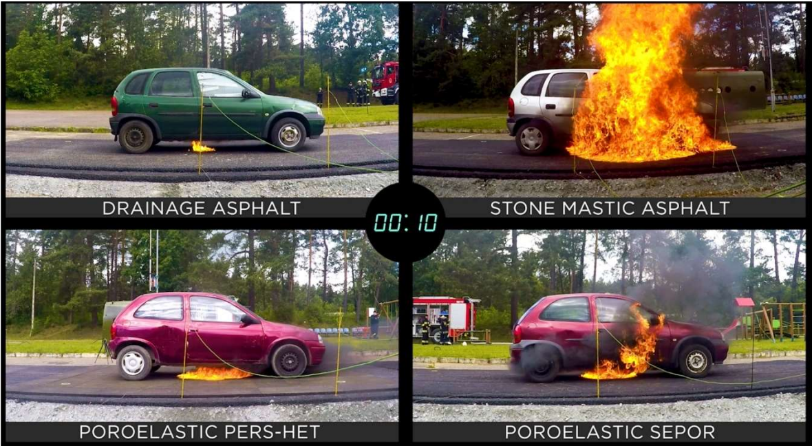
Figure 9. Development of fire 10 s after ignition [27]
