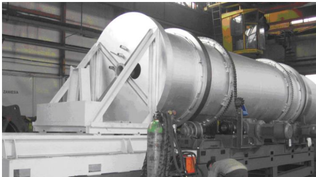
Fig. 3. Detailed view of the rotary pyrolysis chamber.
