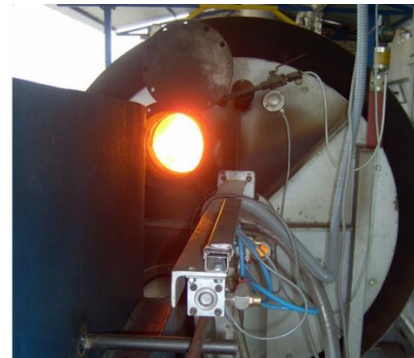
Fig. 3. Detailed view of the rotary pyrolysis chamber.
