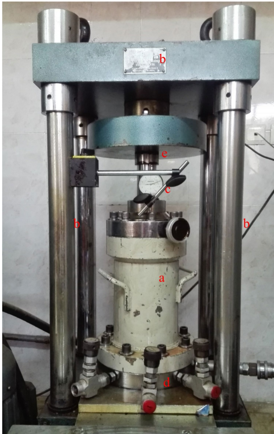
Fig. 5. A three-axis testing machine designed for stone and concrete samples made by Heicoin company. a. Triaxial cell (Sample chamber), b. Hydraulic load frame, c. Dial gauge/displacement sensor, d. Pressure gauges and valves, e. Loading piston.
