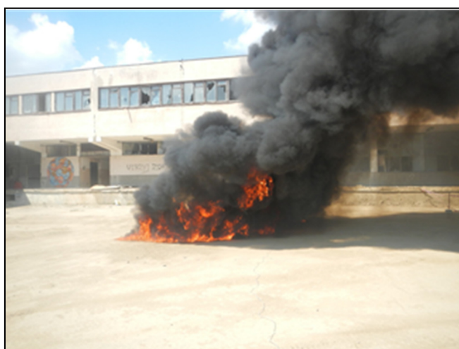
Figure 14. Fire of the 20 L gasoline on dense concrete pavement 15 s after ignition.
