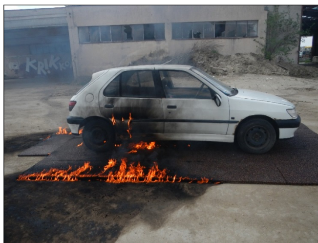
Figure 13. Car fire 260 s after ignition.
