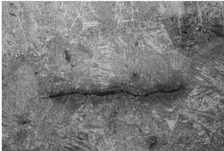
Fig. 5. Exemplary microphotograph of the cold crack in the bainite structure (magnification 200×)
