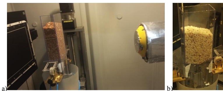
Fig. 1. Experimental set-up a) picture of silo model in X-ray tomography hutch, b) silo model with rice and sorghum mixture.
