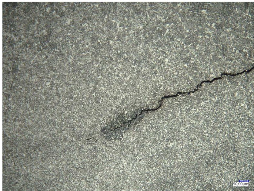
Figure 5. Metallographic microsections of welded joint area (T-tube/straight) engulfing joint material, heat affected zone, native material of the pipeline (a) and magnified region of the identified crack (b).
