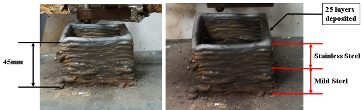
Figure 12. Mild steel and stainless steel bimetallic deposition.
