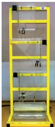
Rys. 1. Kaskada zbiorników Fig. 1. System of cascade tanks
